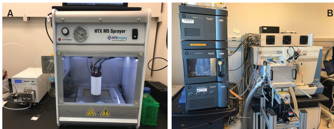
Figure 1. Instruments used in this study. (a) HTX M5 Sprayer; (b) MALDI/ESI injector coupled to Orbitrap Velos mass spectrometer.
